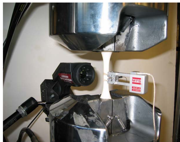
Figure 2. An acrylonitrile butadiene styrene (ABS) copolymer cylindrical dog-bone shaped fatigue specimen mounted in an MTS 810 servo-hydraulic load frame with an MTS model 634.31F-25 axial extensometer for strain-control testing and an Optris Laser thermometer for monitoring temperature generation. [Color figure can be viewed in the online issue, which is available at wileyonlinelibrary.com .]
